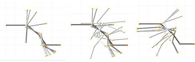
Fig. 9. Snapshots of the 4-link robot under three controls (Left: without time-varying feedback, Middle: with time-varying feedback on cyclic path, Right: with time-varying feedback with a displacement) the starting moment is dark color and the end moment is light color
